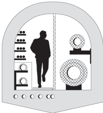
Figure 2. MUT-Section with installed district heating pipes and high voltage cables, based on [3]
